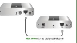
3 Connect the REX to the AC adapter and plug it into a power source.
